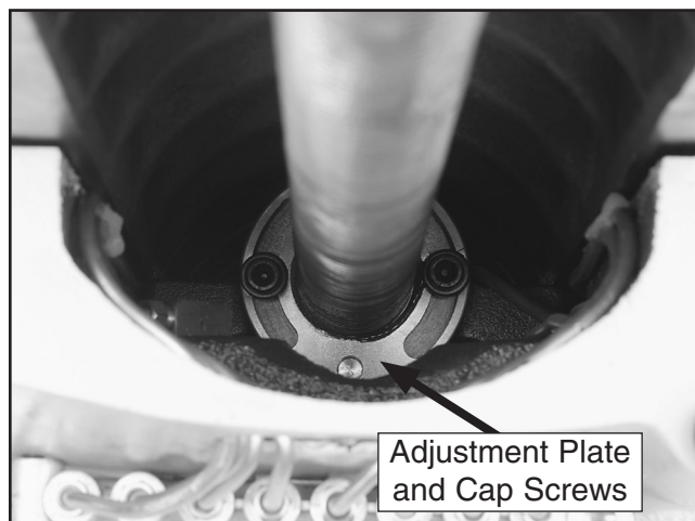
Figure 68. Longitudinal leadscrew adjustment plate and cap screws as seen from the left side of the table.
